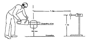
Figure 4: Typical test-site layout and microphone positions: chainsaws (side view)
